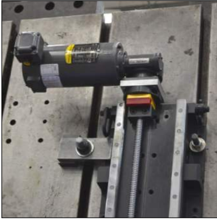
Motor attached to ballscrew on bed
