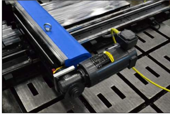
Motor attached to ballscrew on ram
