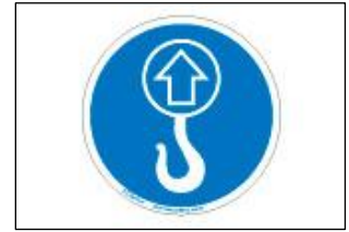
FIGURE 31 LIFTING POINT LABEL 59039
