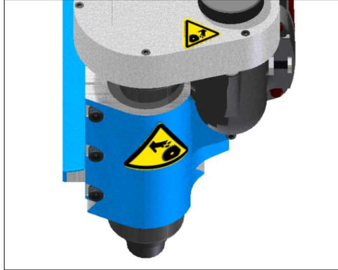
FIGURE 2 LABEL LOCATION ON WELDON SPINDLE
