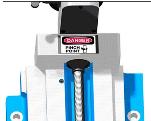
FIGURE 8 FEED DRIVE LABEL LOCATION
