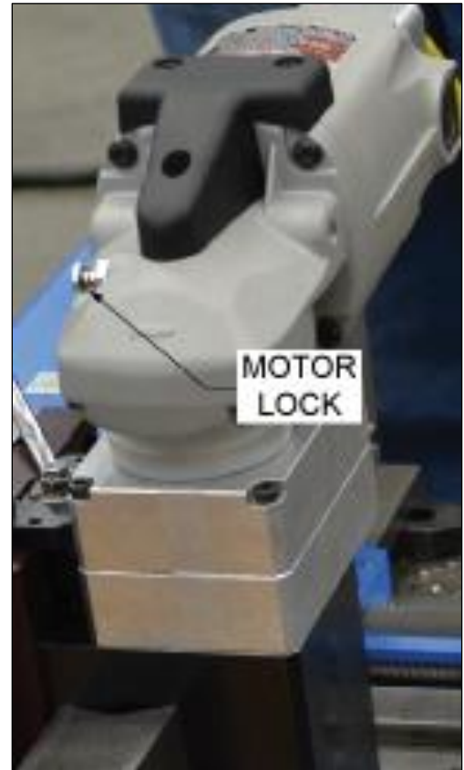
FIGURE 43 ELECTRIC MOTOR LOCK
