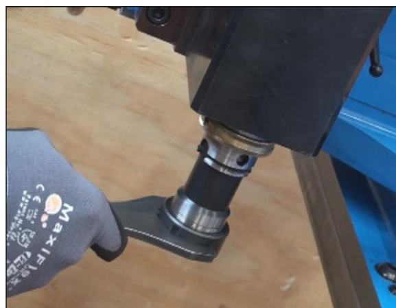
FIGURE 48 HSK END MILL COLLET INSTALLATION
