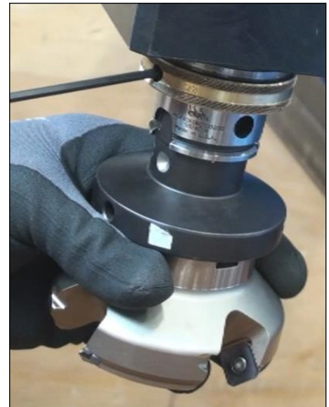
FIGURE 46 REMOVING TOOLING USING ALLEN WRENCH
