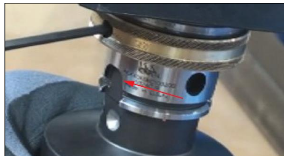
FIGURE 47 DEEP NOTCH IN ONE SIDE OF TOOL HEAD
