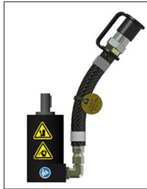
FIGURE 4 HYDRAULIC MOTOR LABEL LOCATIONS
