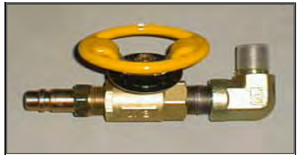
FIGURE 3-17. AIR CONTROL VALVE HANDLE
